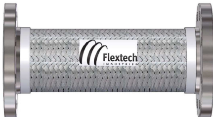
T321 SS Corrugated Hose and SS Braid C/W 150LB 44 W Plate Steel Flanges E/E
